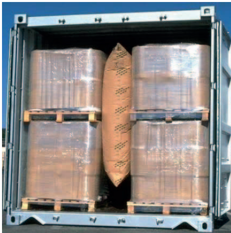
Figure 7.9 – Gap filled with a central dunnage bag
