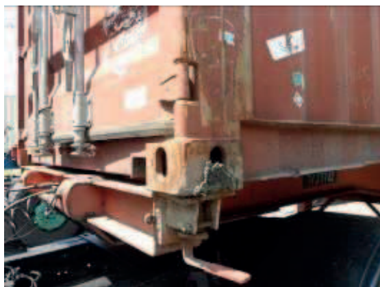
Figure 6.2 – Mud in corner fitting
