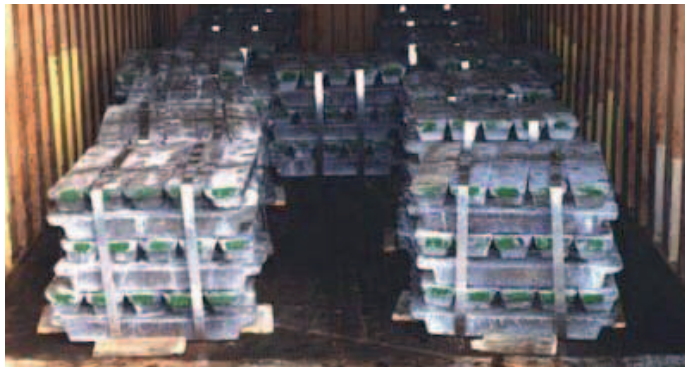
Figure 7.19 – Metal ingots unitized by steel banding (securing not completed)
