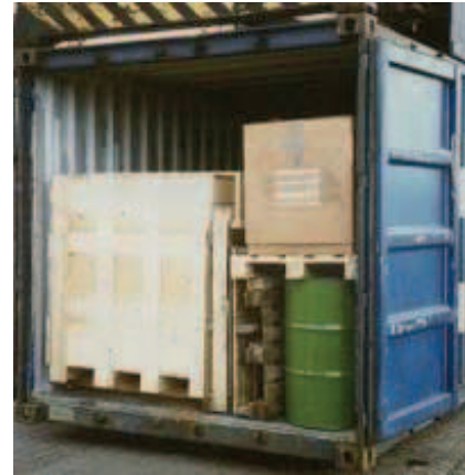
Figure 7.28 – Mixed stow, use of pallets
