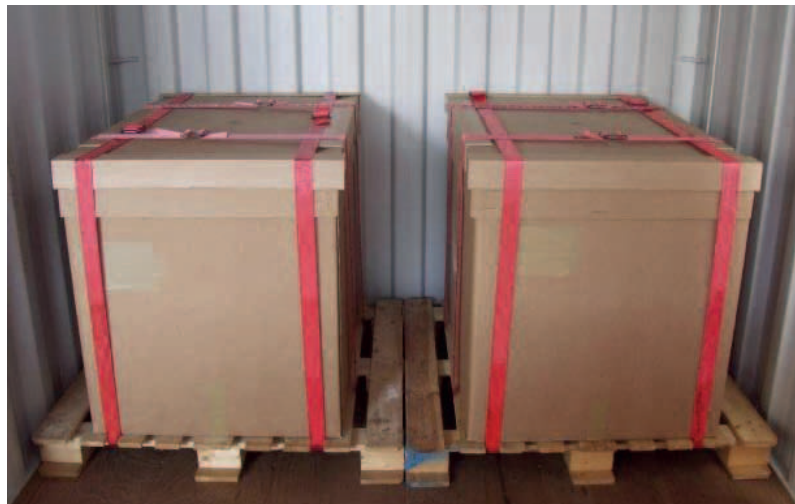
Figure 7.8 – Cargo firmly secured to pallets by textile lashings
