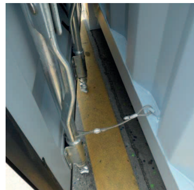
Figure 5.30 – Door retaining strap
