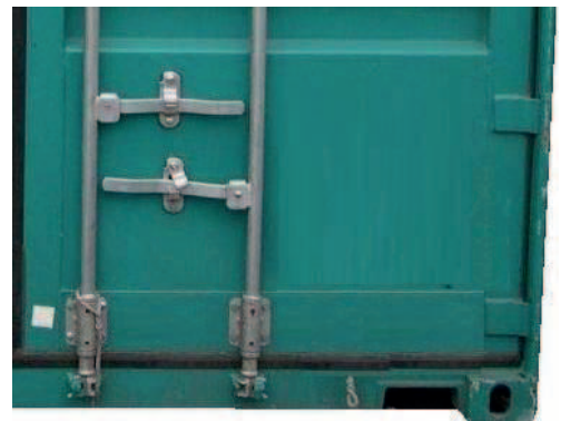
Figure 5.27 – Handles between bars
