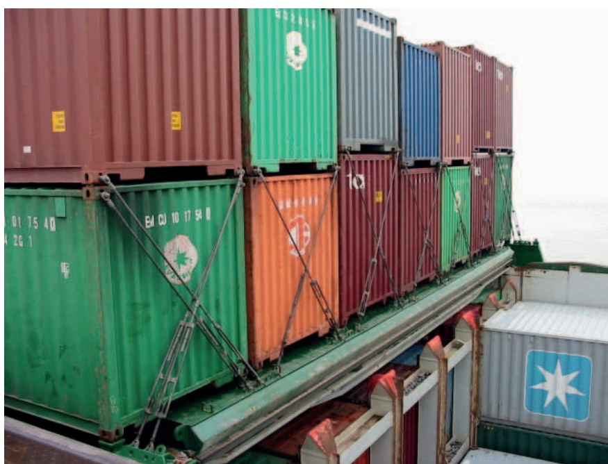
Figure 2.2 – Cell guides and lashing rods on a container vessel
