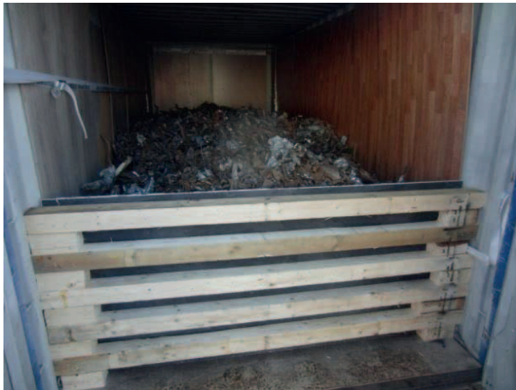
Figure 7.55 – CTU with wall liners and door barrier loaded with scrap
