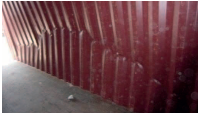
Figure 7.50 – Damaged CTU side wall
