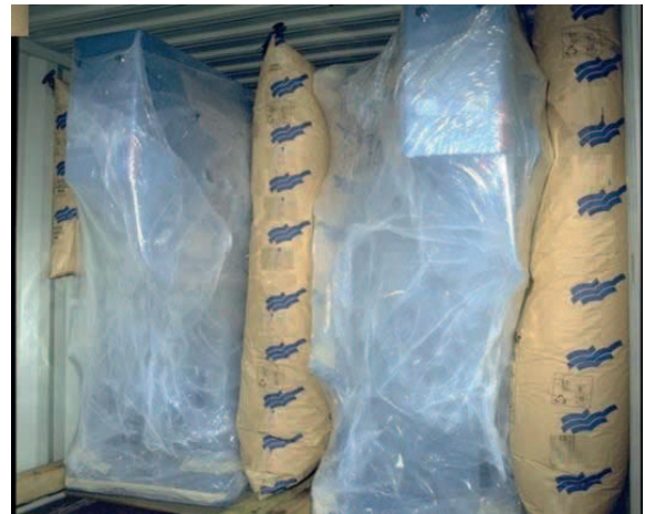
Figure 7.10 – Irregular shaped packages blocked with dunnage bags
