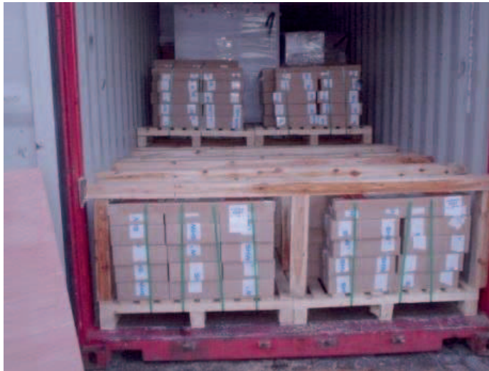
Figure 7.2 – Timber temporary floor
