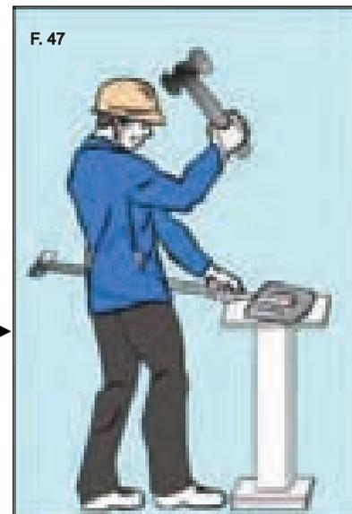
*Figure 47: When need greater force, choose the work station slightly lower than your elbow height.*
