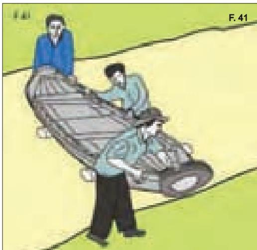
*Figure 41: Use rollers to move heavy objects over short distances.*
