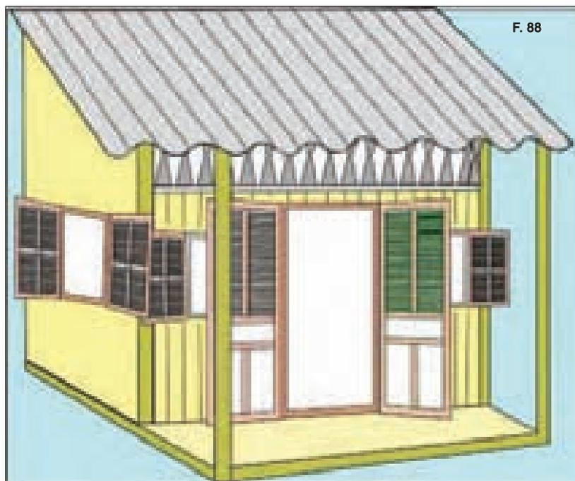
*Figure 88: Open more windows and doors, remove obstacles that prevent natural ventilation.*
