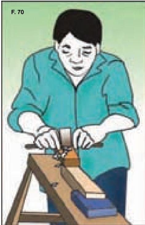
*Figure 70: A low-cost fixture device made of wood to hold the work pieces*
