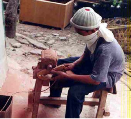
Photo 1.2: Grinding operations produce a lot of dust in the shoe manufacturing. Photo source: ILO-IPEC Footwear Programme.
