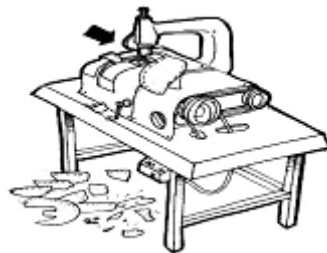
Figure 16.2: Skiving machine for material thinning. Moving machine parts, like the belt in this skiver, should be properly guarded or enclosed. Figure source: ITB and ILO-IPEC Footwear Programme.
