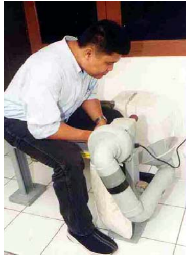
Photo 1.3: A grinder equipped with a dust bag, guard to protect eyes, and seat was developed by the Bandung Technology Institute (ITB) in collaboration with the ILO-IPEC Footwear Programme.
